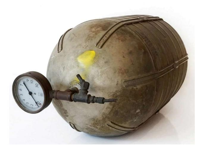
A visit to the local WalMart provided a Nitro Kit from the car accessory aisle. To save time with plumbing, the plane's smoke system was removed and the plumbing utilized for the gases.
