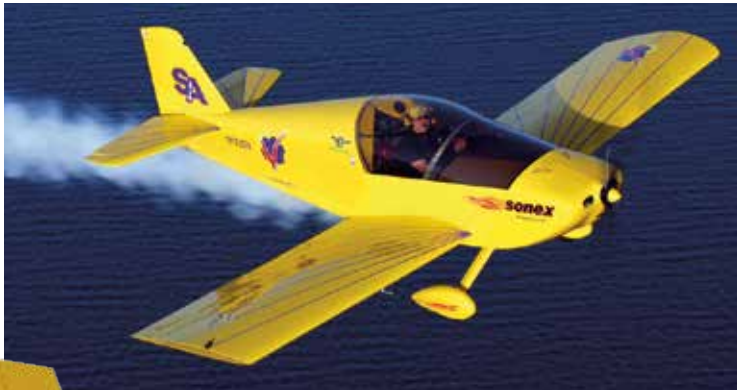
The company demonstration Sonex Sport Acro (SA) has a smoke system (always a plus for photo ops and fly-bys) and a 100-hp AeroVee Turbo engine.
