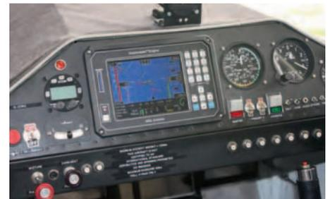
Panel is fitted with MGL Avionics 'glass cockpit'.
