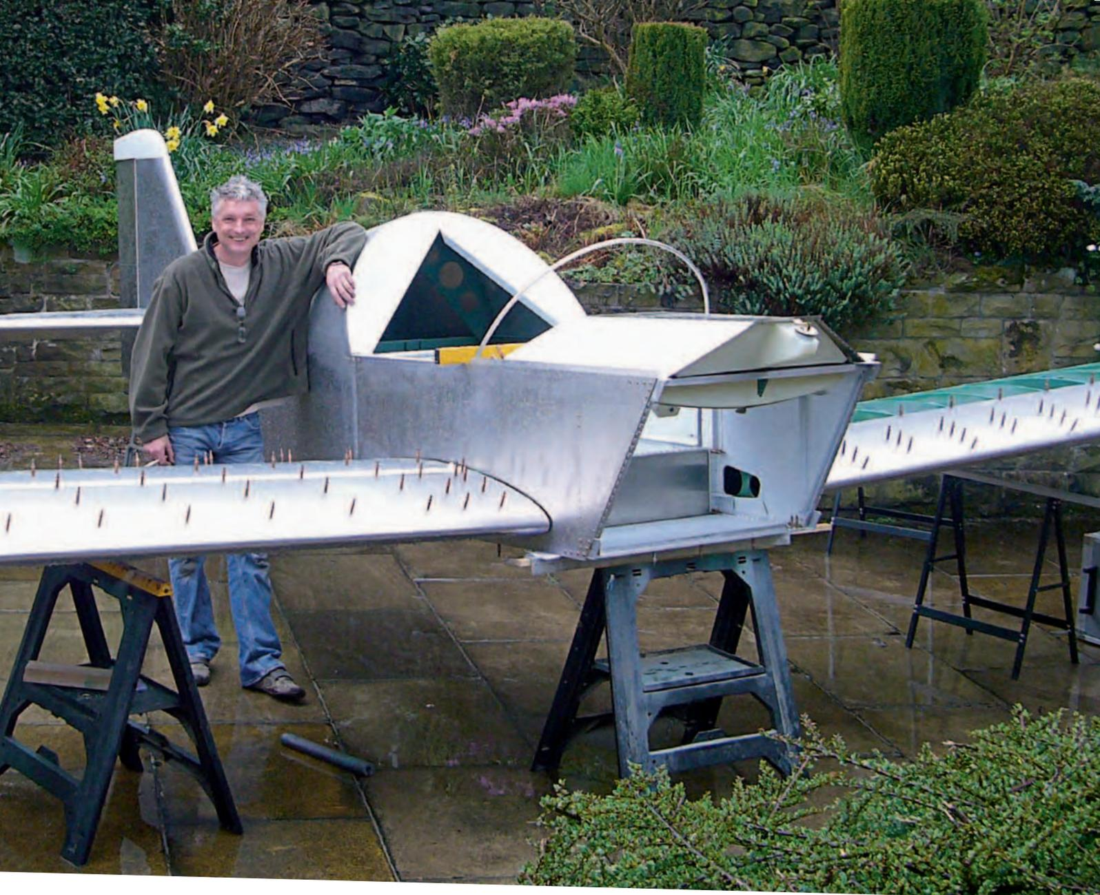
The kit arrived in September 2007 and I drove to Sandtoft in a pick-up truck to collect it. I had decided on a tricycle undercarriage with dual sticks, and plumped for the AeroVee engine. My budget for the entire project was £25,000 and that wouldn't stretch to the Jabiru 3300 engine that Mike had installed in his prototype build.
