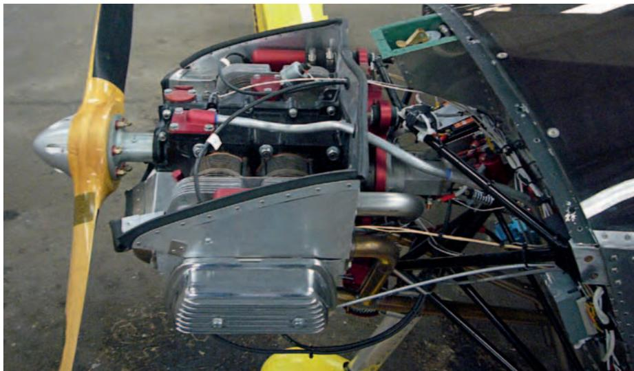
Four-cylinder air-cooled AeroVee engine is light weight and economical to buy and operate.
