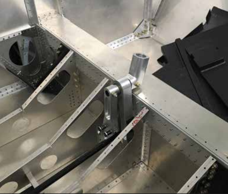
The seat ribs have been changed and beefed up, with the new seat pan riveted in place. The center stick is mounted in a billet-machined hinge assembly, and is much simpler than dual sticks.
