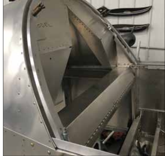
The rear cabin bulkhead and cross brace have been modified to allow a more reclined seat back position, thus providing more space in the cockpit.
