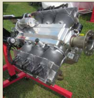
The 120-hp direct-drive Jabiru 3300 is often used to power Sonex aircraft.
