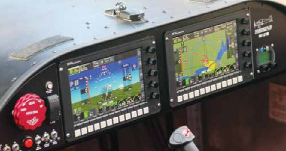
The panel on the B-Model is much larger, allowing for full-sized EFIS screens to be installed.
