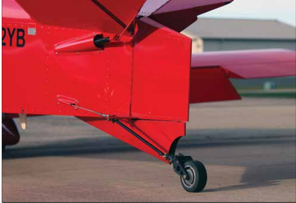
Control-rod exit fairings are now made out of vacuum-formed plastic, a nice kit addition that saves hours of metal forming by builders.
