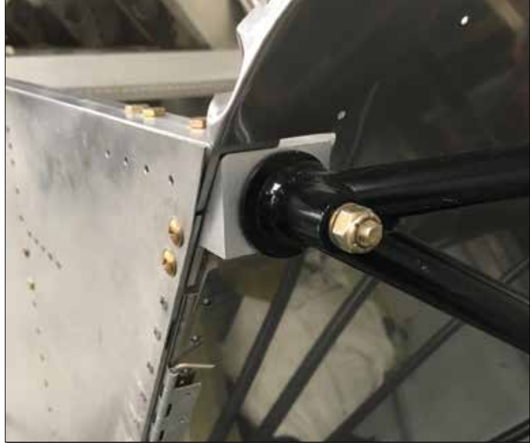
The engine-mount attach points are beefed up over previous designs, and allow larger engines than the original models.
