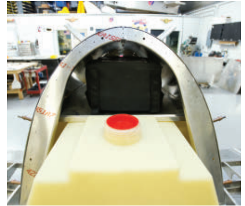
A molded fuel tank is located behind the pilot seat.
