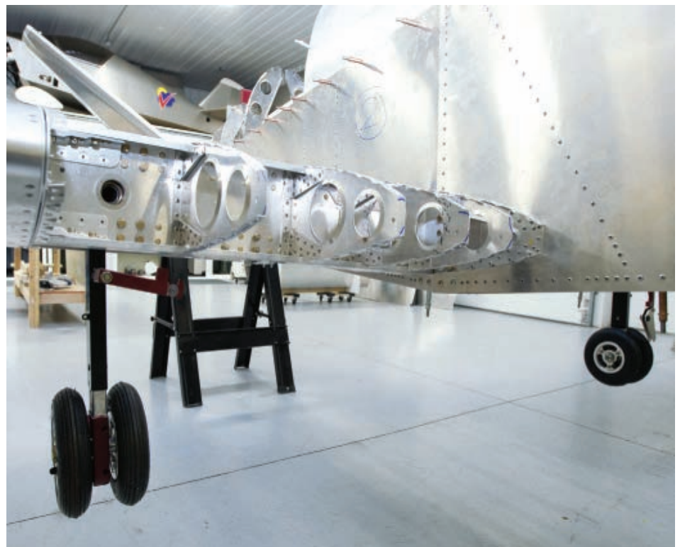
Retractable main gear is a new feature in the SubSonex, and dual main wheels are extremely rare in light airplanes of any type.
