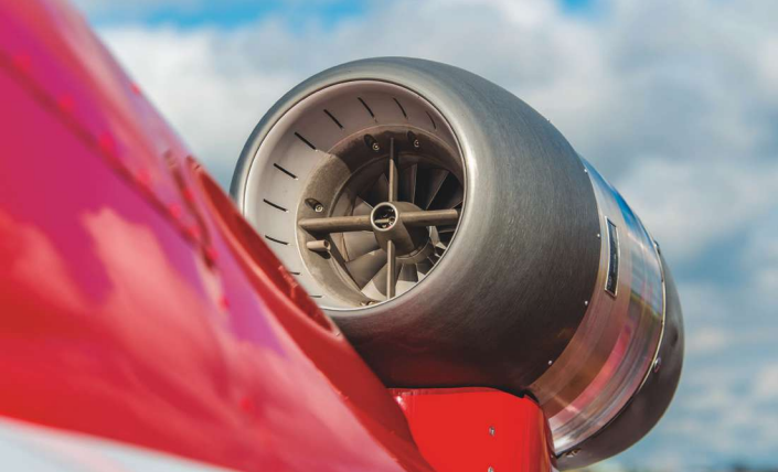
The Czech-built PBS engine only weighs 44 pounds yet puts out 250 pounds of thrust.
