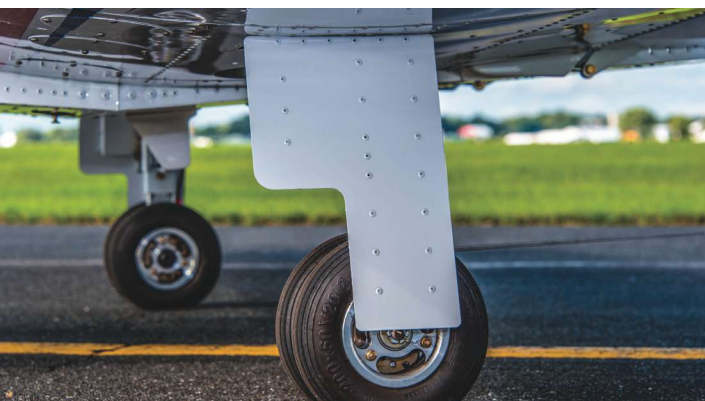
The landing gear system is pneumatically operated by an electric pump behind the pilot's seat.
