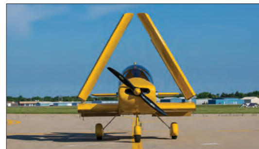
The magic beneath the skin of the folding wing—a rugged hinged spar allows the outer wing panels to fold for compact storage.
