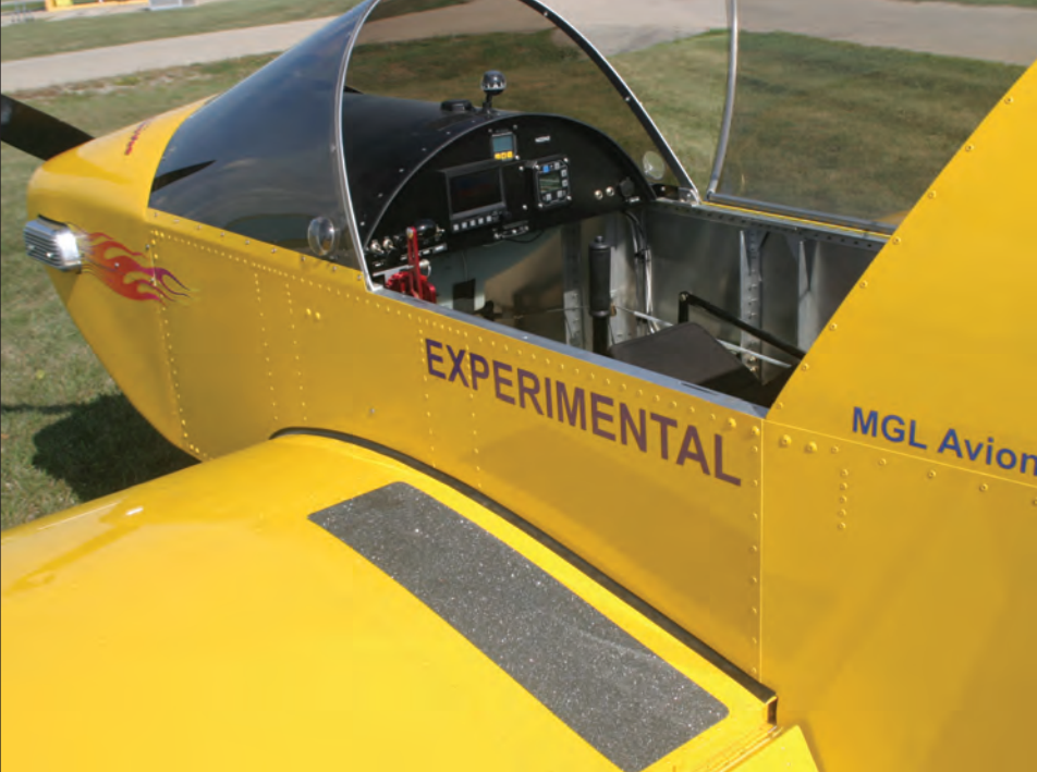
The swing-over canopy provides easy access to the cockpit.
