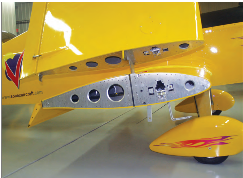
The wing-fold mechanism allows automatic connection of the aileron pushrods.
