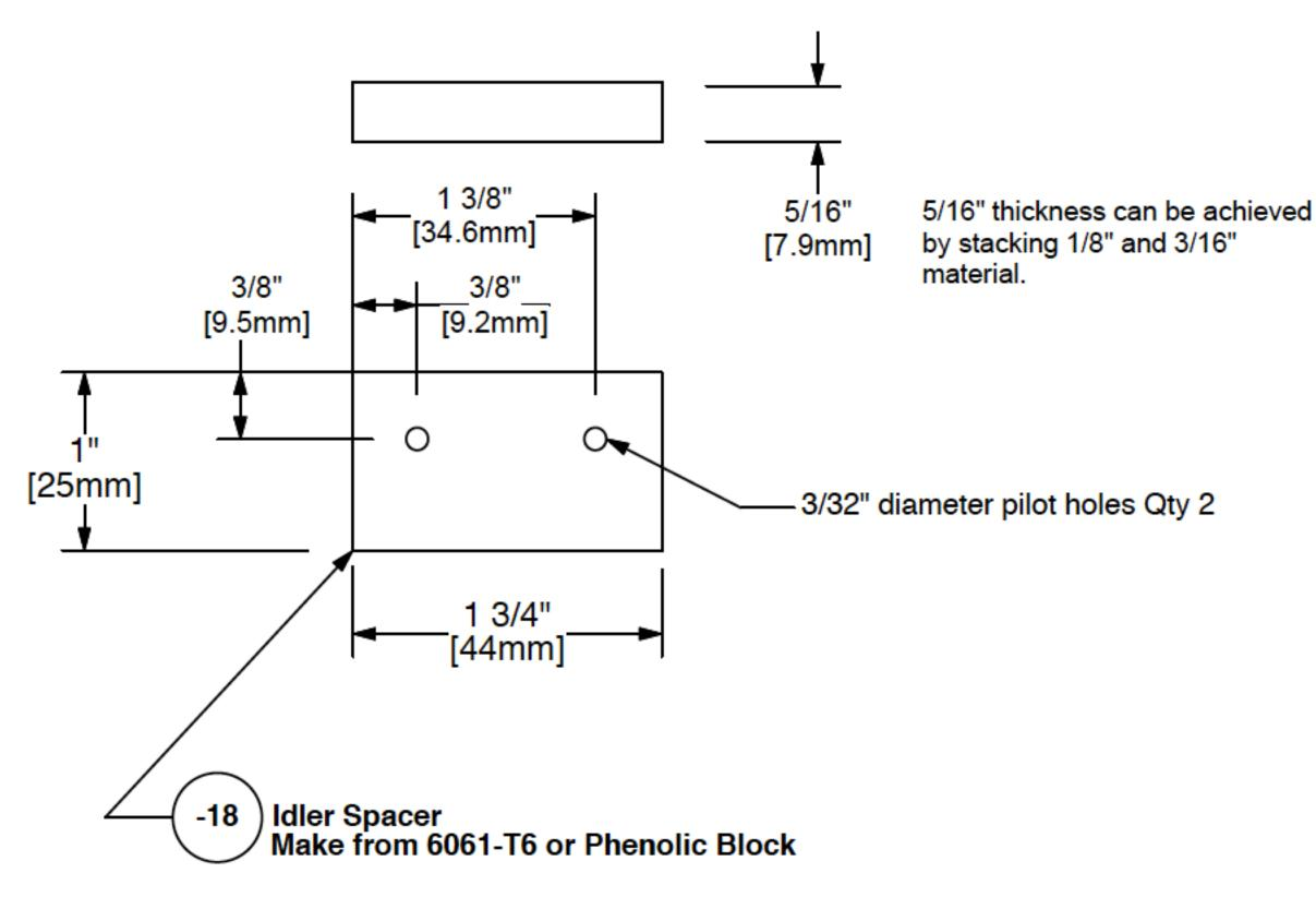
Note: The 5/16" thickness can be achieved with a combination of 1/8" and 3/16" thick 6061-T6 aluminum or phenolic block. You will need 2 parts that are 1/8" thick and 2 parts that are 3/16" thick.
