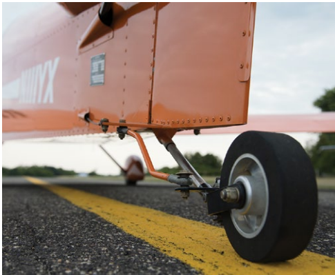
The tail wheel has direct steering—no springs.
