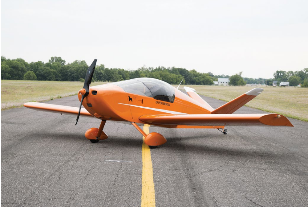
Designer John Monnett’s Waix has a V tail with a lower rudder, making it a “Y” tail.
