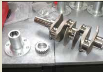
The AeroVee engine is available as a kit, and the crankshaft can come with the prop flange pre-assembled or in a DIY package (shown here).
