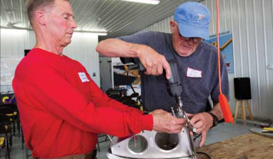
Chuck Sheldon holds while his building buddy Richard Nichols drills rivet holes in the spar cap.
