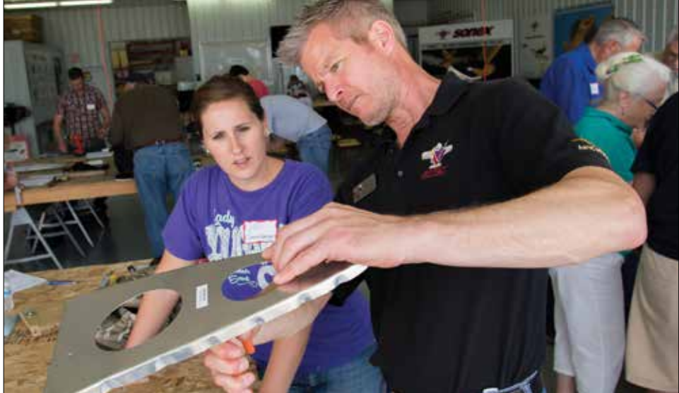
Sonex technical guru Kerry Fores shows Jill Steenberg how to flute her nose rib.
