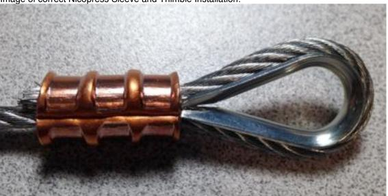
Note that a cable installed flush with the end of the Nicopress Sleeve is serviceable and does not present a safety hazard.
