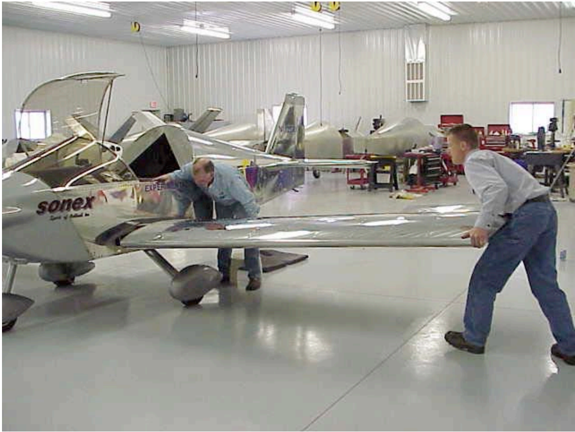
Step 8: Push the spar pins into place.
