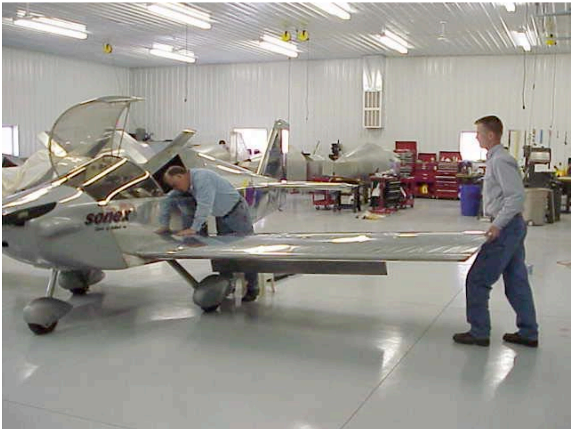
Step 8: Push the spar pins into place.
