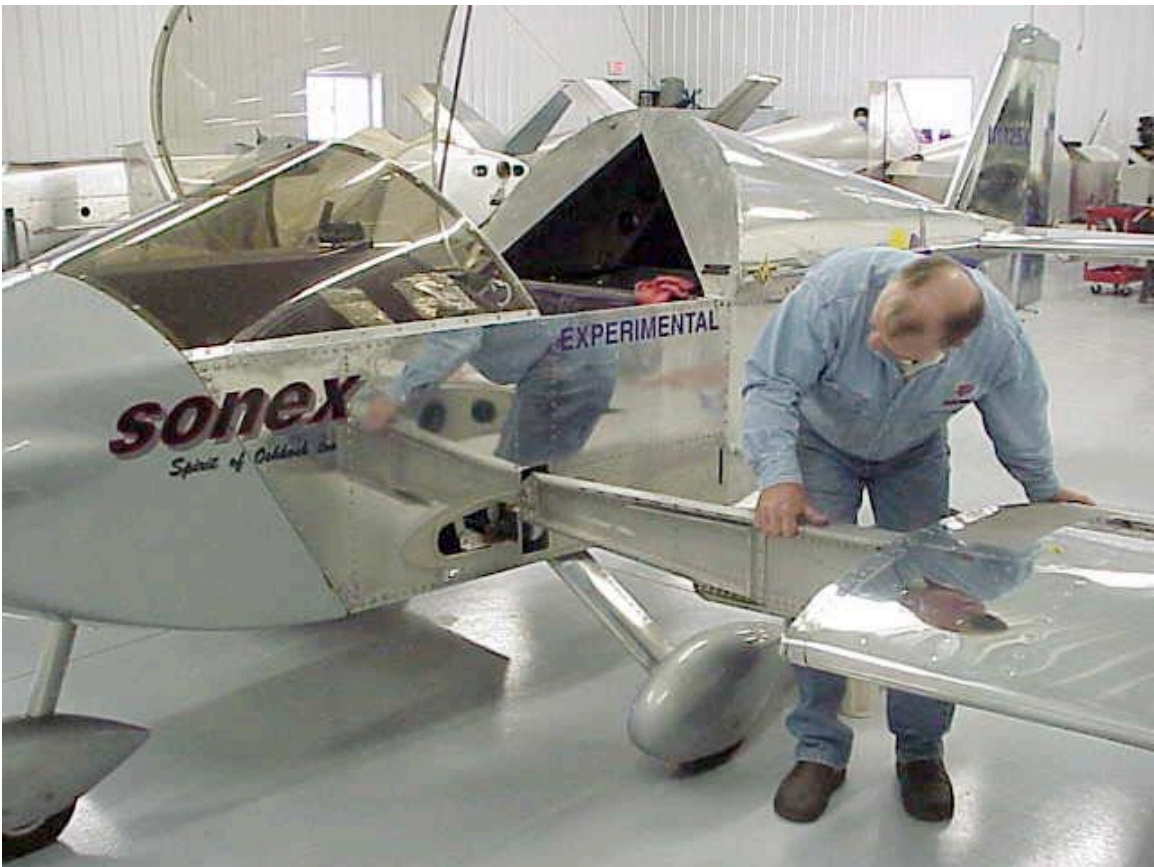
Step 6: Slide left wing partially into the spar tunnel.
