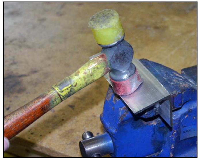
This extrusion's angle is being reduced by striking the unclamped leg with a rubber mallet. Pad the vise jaws to reduce marring clamped leg.
