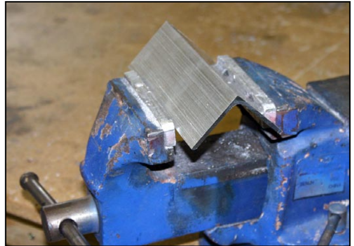
This extrusion's angle is being reduced by being squeezed in a vise. Pad the vise jaws to reduce marring of the part.
