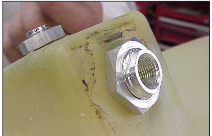
The Oops fitting installed.
