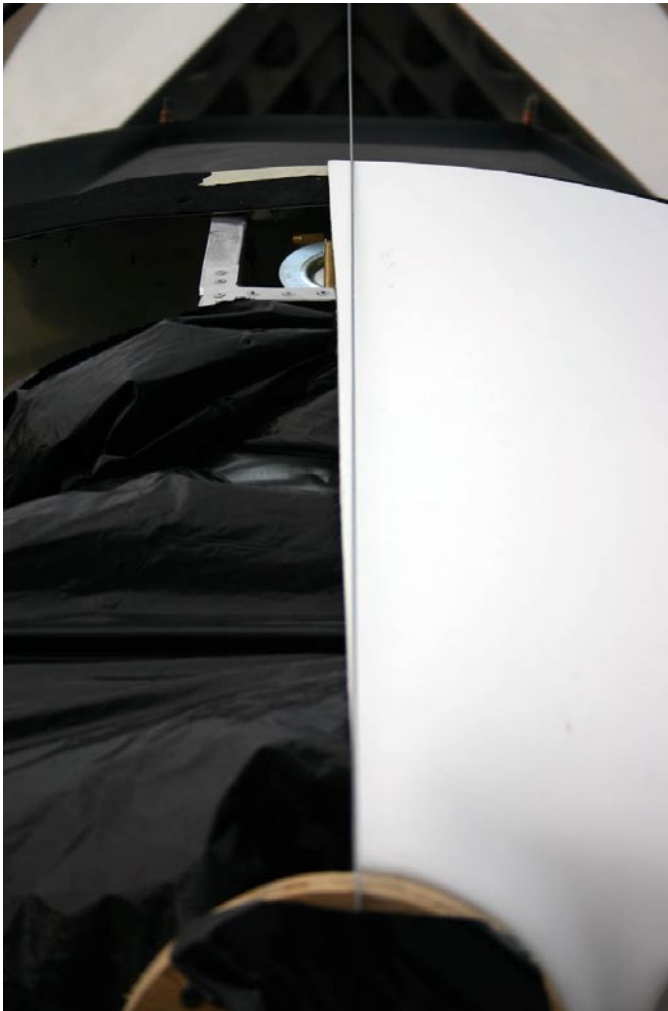
A string stretched from the centerline of the prop hub to the centerline of the turtledeck identifies the centerline (trim line) of the upper cowl seam.
