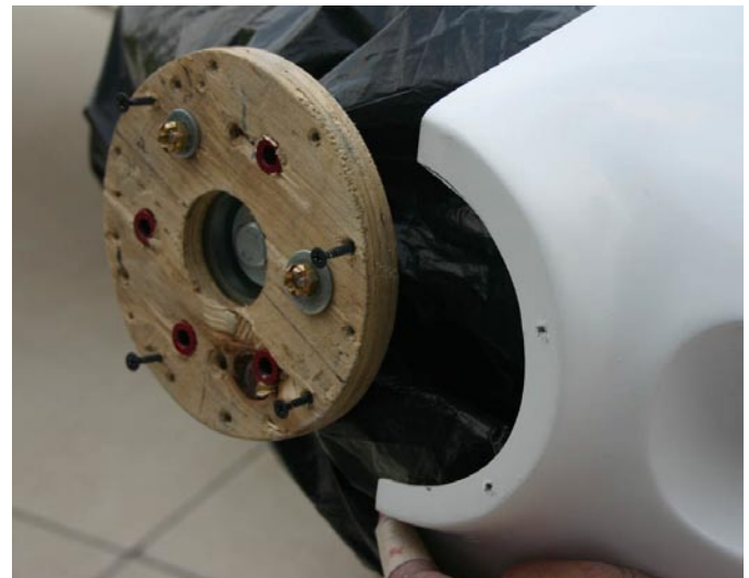
The opening for the prop hub must be cut to eliminate interference between the cowl and the flange of the prop hub.
