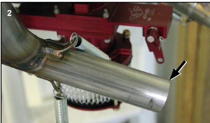
*Trim the end of each exhaust manifold (arrow) as needed to get the exhaust extensions to exit the cowl in the desired location.*
