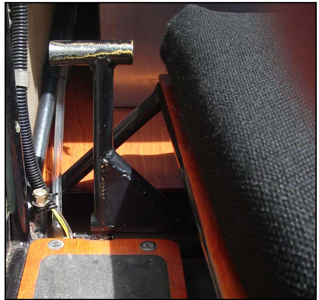
Rear Rudder Pedal Reinforcement
