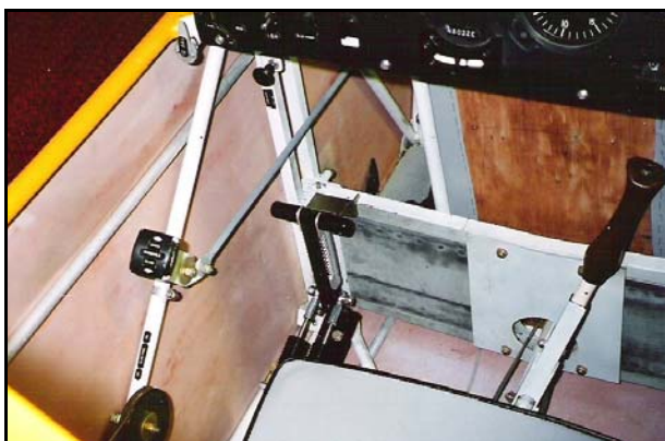
Here are the master cylinder levers in the normal operating position.
