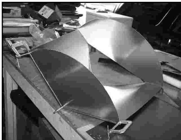
Initial Fit-up Note the flanges at each of the joints.
