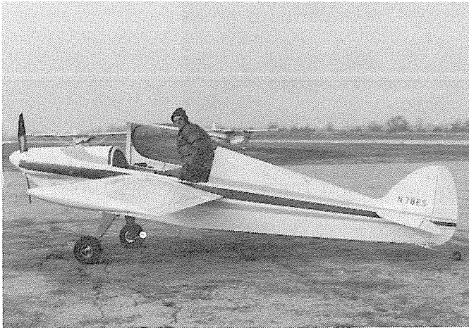
Sonerai II 78ES made by Edward J. Sterba, 106 Center, Fox River Grove, Ill. Test flight; November 25, 1978. Construction began April, 1977. Building time approx. 1000 hours. Engine 1850 cc V.W. 5244 Rehm prop. 1979 Best Sonerai II
