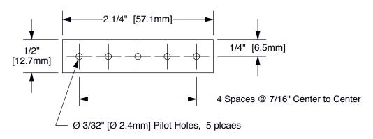
Repair Plate - .032" Thick 6061-T6 Aluminum
