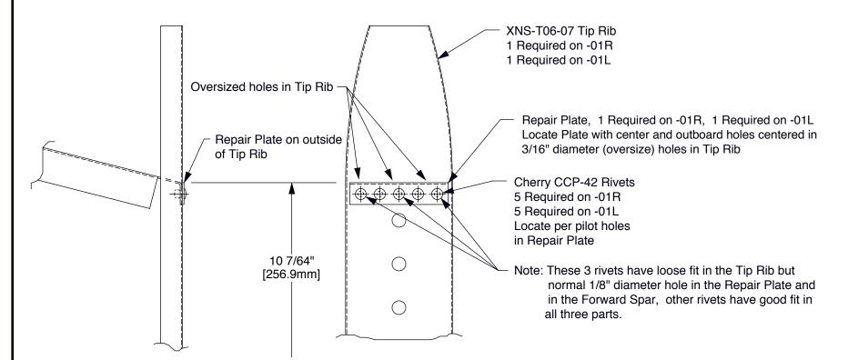
Reference XNS-T05 Stabilator Substructure
