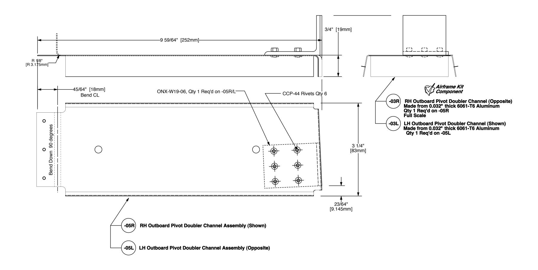
ONX-W20-05R/-05L Pivot Doubler Channel Assembly with new Outboard Pivot Doubler Channel Supplied with all Onex Kits since September 15, 2012
