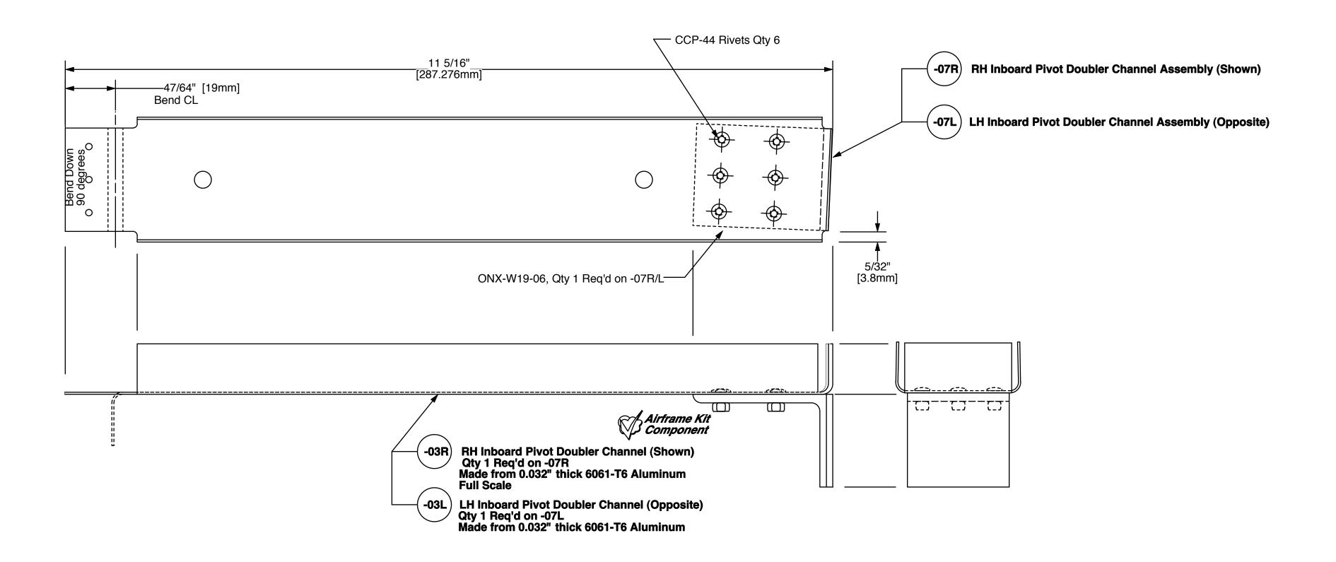
ONX-W19-07R/-07L Pivot Doubler Channel Assembly with new Inboard Pivot Doubler Channel Supplied with all Onex Kits since September 15, 2012
