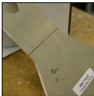
The bend centerline is marked on this Sonex spar fitting.
