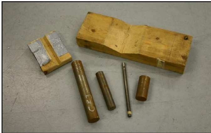
Homemade wood V-blocks and rods of various diameters. While solid steel rods are shown here, wood dowels and steel pipe would also work.
