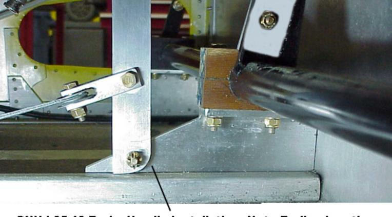
SNX-L05-12 Brake Handle Installation. Note Radius location which serves as the forward stop for the brake.
