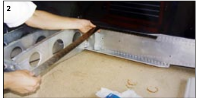
A carpenter's square works well for setting the rear spar's position relative to wing station 0.0. (See step 2)
