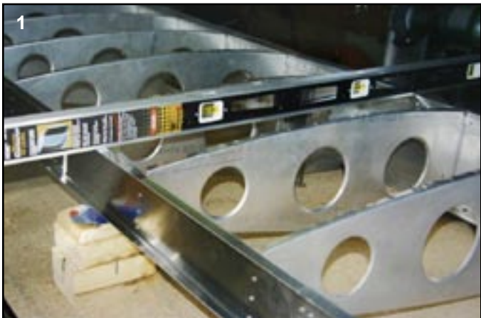
The spars are shimmed off the workbench as needed to get them level at both the tip and root.
