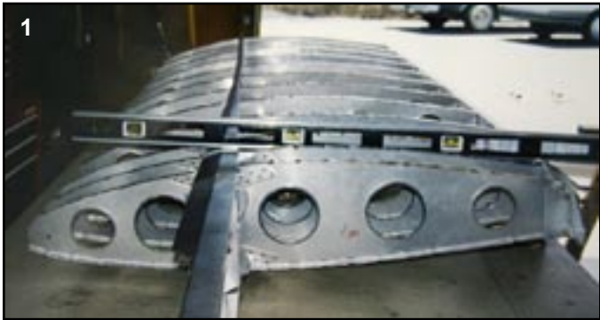
While two levels speeds the job, a single level can be used, checking each end of the wing structure for level.
