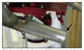
Trim the end of each exhaust manifold (arrow) as needed to get the exhaust extensions to exit the cowl in the desired location.
