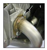
2. Slide an extension pipe onto each manifold. It may be necessary to shorten the length of the exhaust manifold if the extensions interfere with the firewall. **Do not shorten** the expanded portion of the extension pipes.
