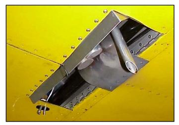
This photo shows the standard outlet for a 2-into-1 exhaust fitted to a cowl without pre-molded tunnels. The cut-out measures 4" x 12.5". No additional cowl outlets are needed for cooling air. The small tube in this photo is the oil breather.
