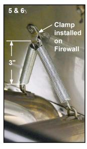
7. Trim the ends of the exhaust pipes to final length. The pipes must be long enough to ensure the exhaust gases exit the cowl, yet pipes which extend too far below the cowl will add drag and reduce your airspeed.
