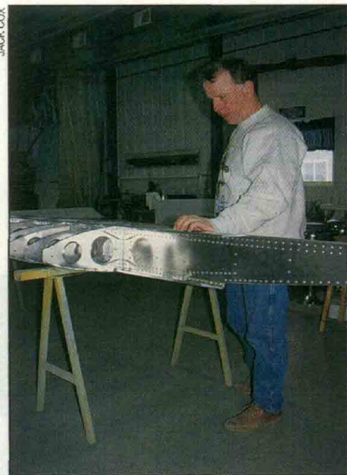
John Monnett provides perspective to show the massive spar carrythrough for one of the Sonex wings.
