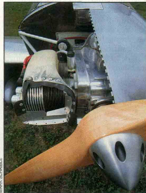
The Sonex cowling splits vertically. Note the machined aluminum spinner. It looks good and allows visual inspection of the prop bolts.
