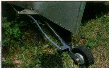
The Sonex has a direct steering tailwheel (no springs) like those Steve Wittman used on his Tailwinds and racers.
