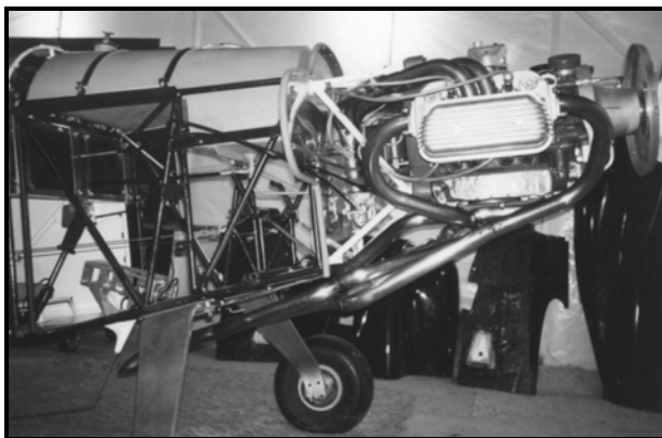
Here's a pretty good view of the "complete" (meaning extended 4-into-1, matched-length) exhaust system. I suspect that it was designed to increase the horsepower output, and to help deal with the strict European noise regulations. You can also see the Monnett SuperVee prop hub/extension.
