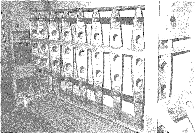
Wing in the jig ready for skinning.
